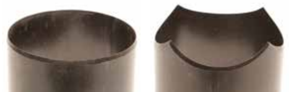
Outside sharpened: push up native soil
